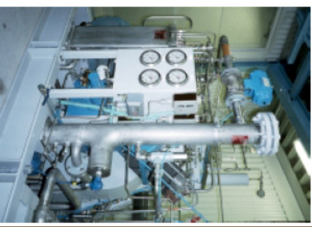
A compact unit that scrubs and compresses biogas for use as an alternative motor fuel
