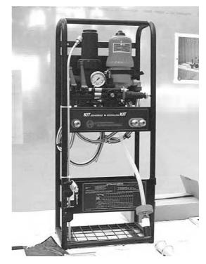
Figure 6.2 This weed control steamer is used to kill weeds without the need for conventional weedicides.
