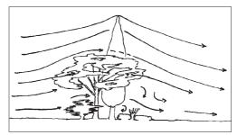
Figure 9.1 A dense windbreak
