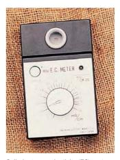
Soil electro conductivity (EC) meter. The EC reading indicates how fast electrons are flowing in the soil. The faster the flow, the higher the nutrient availability of the soil.
