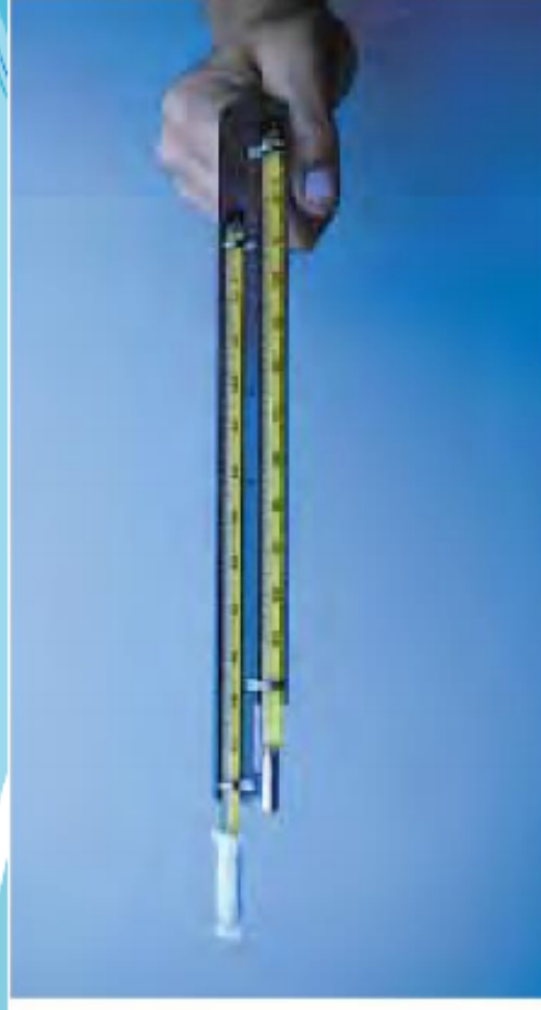
FIGURE 4.9 The sling psychrometer.
